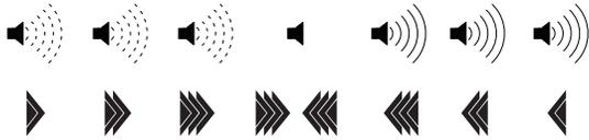
In this mode the unit will display directional arrows to the conductor. The audio indicator will provide a solid tone on one side of the conductor and a pulsed tone on the opposite side of the conductor. When the unit is centered in the electromagnetic field the tone will null and the depth will briefly display at the top of the LCD. This mode is gain independent.
