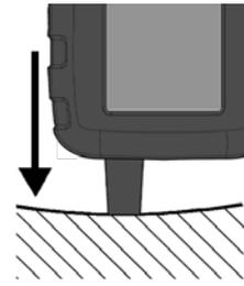
Rubber sleeve in contact with the surface. Hold steady.
