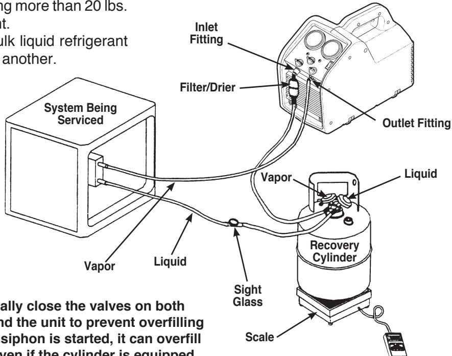
**⚠ WARNING :** Manually close the valves on both the storage cylinder and the unit to prevent overfilling the cylinder. Once the siphon is started, it can overfill the storage cylinder, even if the cylinder is equipped with a float level sensor. The siphon can continue even when the unit is turned off.
