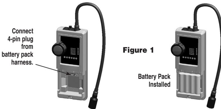
4. Reinstall the battery cover and screw.
