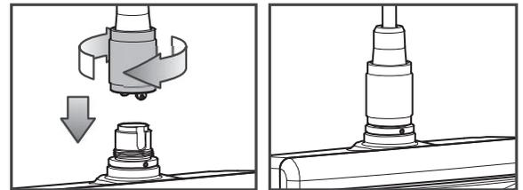
You can now remove the protective red rubber cap from the camera-tipped end of the probe. It is good practice to replace the cap whenever the probe will not be used for a while.
