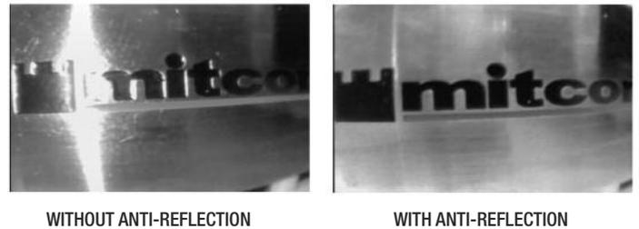
You can also use the anti-reflection function to remove glare created by the P16181HP's mirrored viewing tip (see the next section of this manual for installation and alignment instructions). The pair of images at right illustrate the net positive effect.
