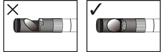
Before using the DCS2000 system, carefully read the Operating, Maintenance & Troubleshooting Tips section of this manual on p. 13 to understand how to use a borescope probe properly and avoid using it improperly. To protect the delicate camera-tipped end of the P16181HP probe, reinstall the rubber lens cap after each inspection session. Don't forget to remove the cap from the tip of the probe before using it again.
