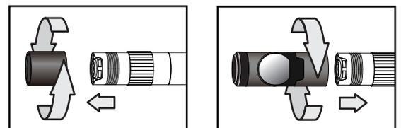
4. Screw the mirrored viewing tip onto the camera head (Callout 2) by turning it clockwise, as shown by the image at right at the bottom of the previous page. Keep turning until the viewing tip is as far from the probe tip as possible. In this position, it can rotate freely.
