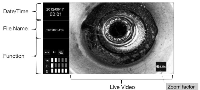
**To stop recording**, press the  $\text{⏏}$  button again. This returns the DCS2000 to Preview mode and replaces the red running clock by the file name of the video clip for 1 minute and 30 seconds (1:30). Like photo files, video files begin with the letter PICT; unlike photo files, video files have the suffix ".AVI".
