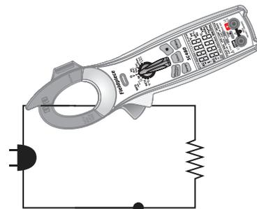
Amps AC (AAC), Frequency (Hz) through the clamp and Inrush AAC current is measured in the VAC/AAC/Hz switch position shown above.
