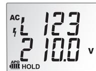
Simply swap any two lines to change the direction. You can verify this by performing the test again.
