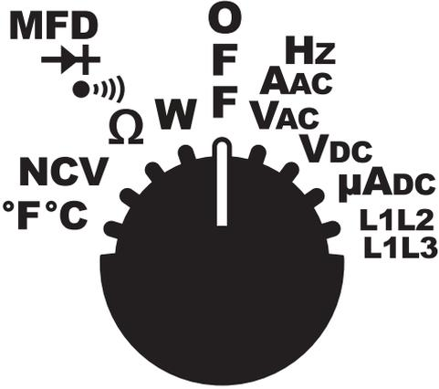
The SC480 is loaded with the measurement parameters essential for HVACR professionals. Select the parameter on the dial you want to measure with the rotating selector switch.
