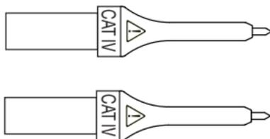
Test probes  $\varnothing$  2 x 15 mm (one red and one black)
