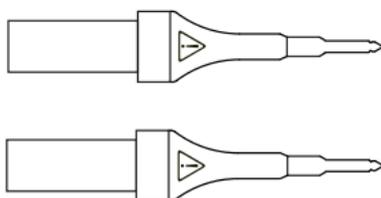
Test probes  $\varnothing$  4 x 15 mm (one red and one black)
