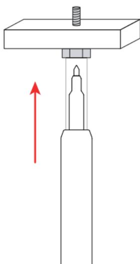
To perform a test, place the test probe on the object to be tested and press to slide the protective cover.
