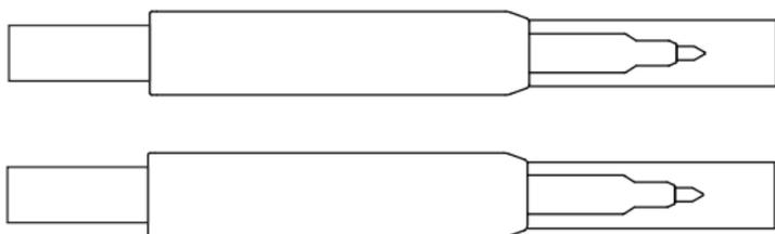
Red IP2X test probe Ø 4 mm (one red and one black)
